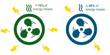
Replacing a conventional motor with a new ECM saves energy through reduced motor friction and heat losses, as well as integrated speed control that matches the motor speed to the system load.
