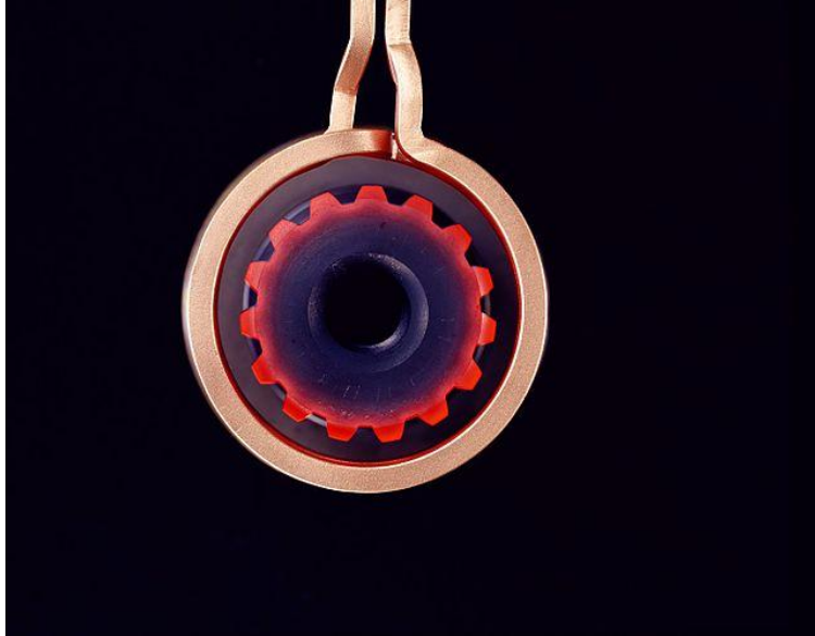
Heating gear teeth with induction heater
