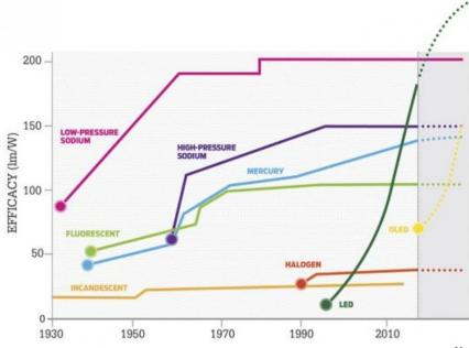
Figure 1: Efficacy trends of common streetlight luminaires across the years<sup>22</sup>
