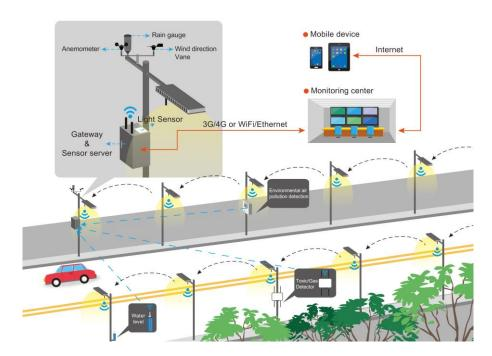
Figure 1: Example of an intelligent streetlighting network with various sensors that communicate to the CMS and mobile devices<sup>2</sup>
